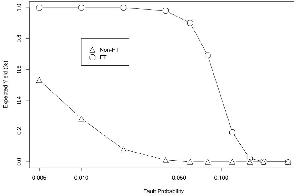
Figure 8: Comparison of yield for non-fault-tolerant and fault-tolerant versions of the BLITZEN chip.
