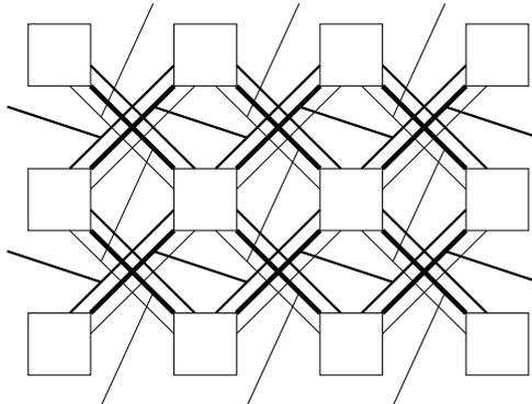
Figure 7: Wiring required for the fault-tolerant network, with Inverse Adjacency Domain  $[i, j]$ ,  $[i + 1, j]$ , and  $[i, j + 1]$ .
