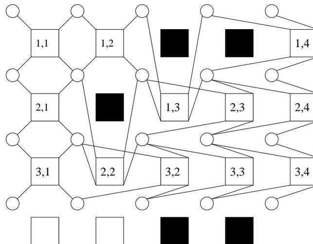
Figure 3: Example of reconfiguration, using one extra row and one extra column of processors. The indices represent logical processors.
