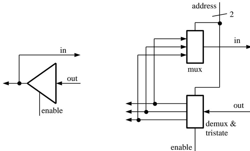
Figure 6: (a) I/O buffer at each corner of each processor for the non-fault-tolerant BLITZEN. (b) Architecture of a switch at each corner of each processor for the fault-tolerant version of BLITZEN (IBN).
