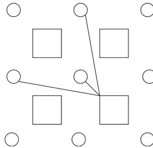
Figure 2: Possible connections between a corner of a processor and three buses
