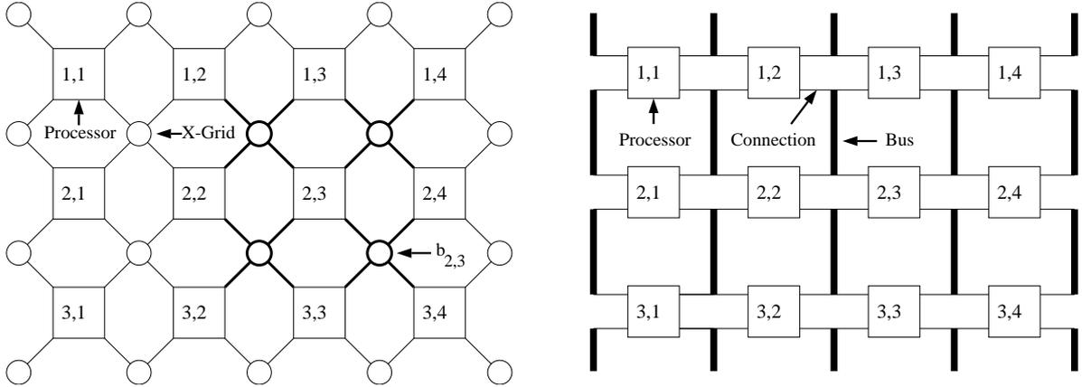
Figure 1: The BLITZEN architecture (processors and X-grid), a) logical view, b) physical construction (processors and connections not drawn to scale).
