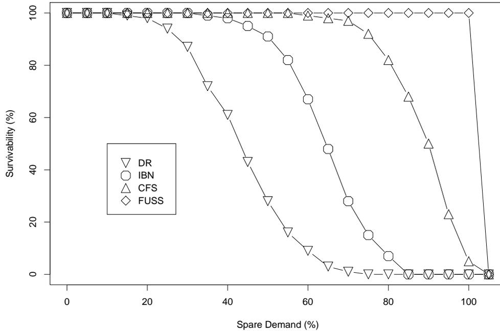
Figure 5: Comparison of survivability of a  $20 \times 20$  processor array, for four reconfiguration methods, including the proposed method (IBN).
