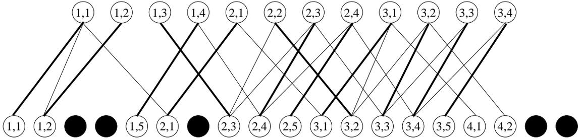
Figure 4: Bipartite graph representing the mapping problem of Figure 3. A logical array of size  $3 \times 4$  must be mapped onto a physical array of size  $4 \times 5$ . An optimal matching is shown by the darkened lines.
