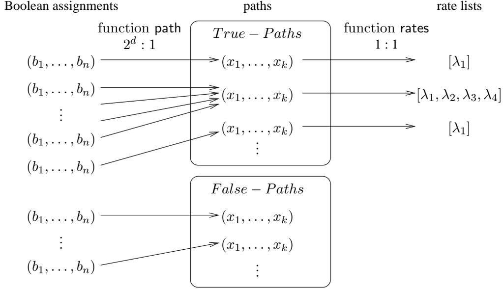
Figure 4.4: Correspondence between Boolean assignments, paths and rate lists
