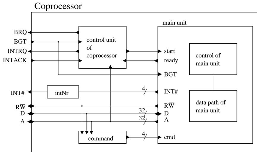
Figure 8.2: Block diagram of the coprocessor
