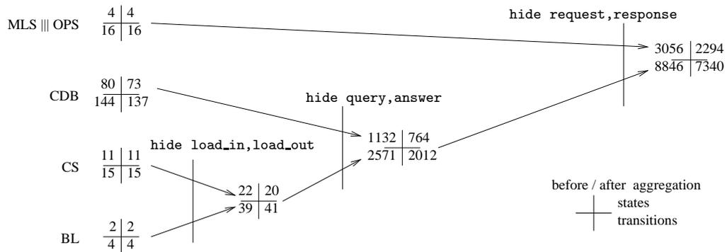
Figure 10.4: Compositional aggregation of the state space of the hospital communication system
