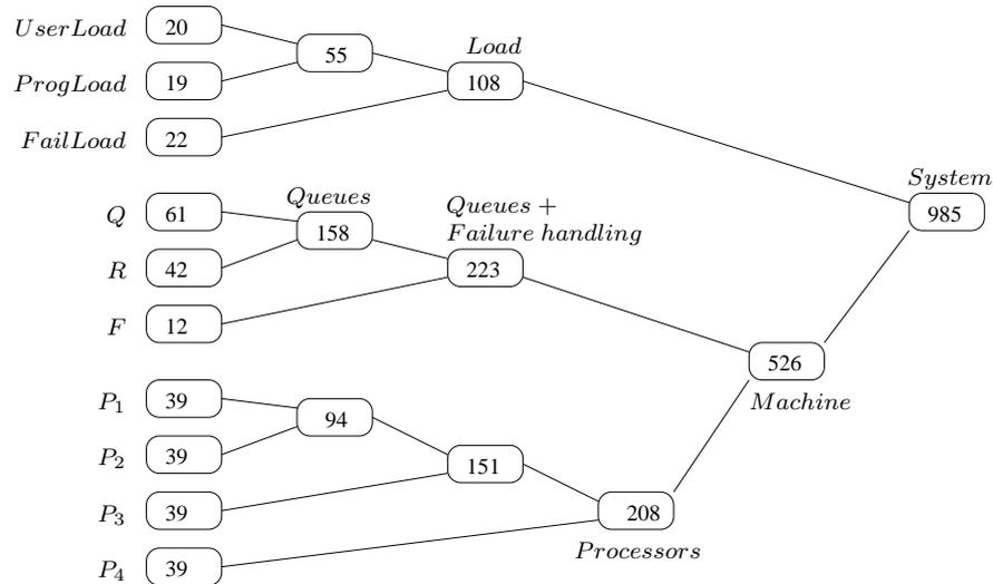
Figure 10.10: Compositional MTBDD construction for the multiprocessor mainframe system: Number of MTBDD vertices (for Markovian transitions)
