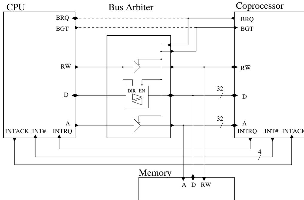
Figure 8.1: Overall configuration, consisting of CPU, coprocessor, bus arbiter and memory
