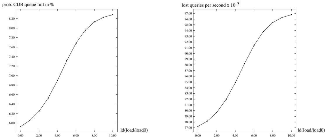
Figure 10.6: Left: probability of the CDB queue being full. Right: rate of lost queries.
