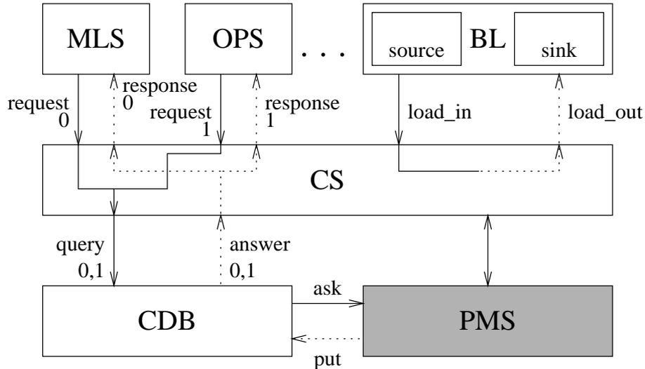
Figure 10.1: The hospital communication system model
