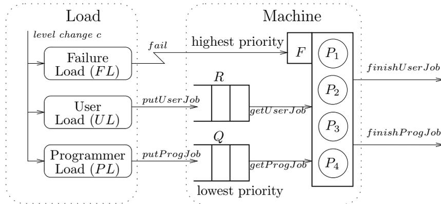
Figure 10.9: Mainframe model structure
