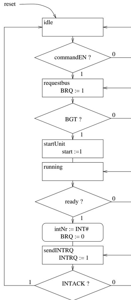
Figure 8.3: State machine of the coprocessor's control unit
