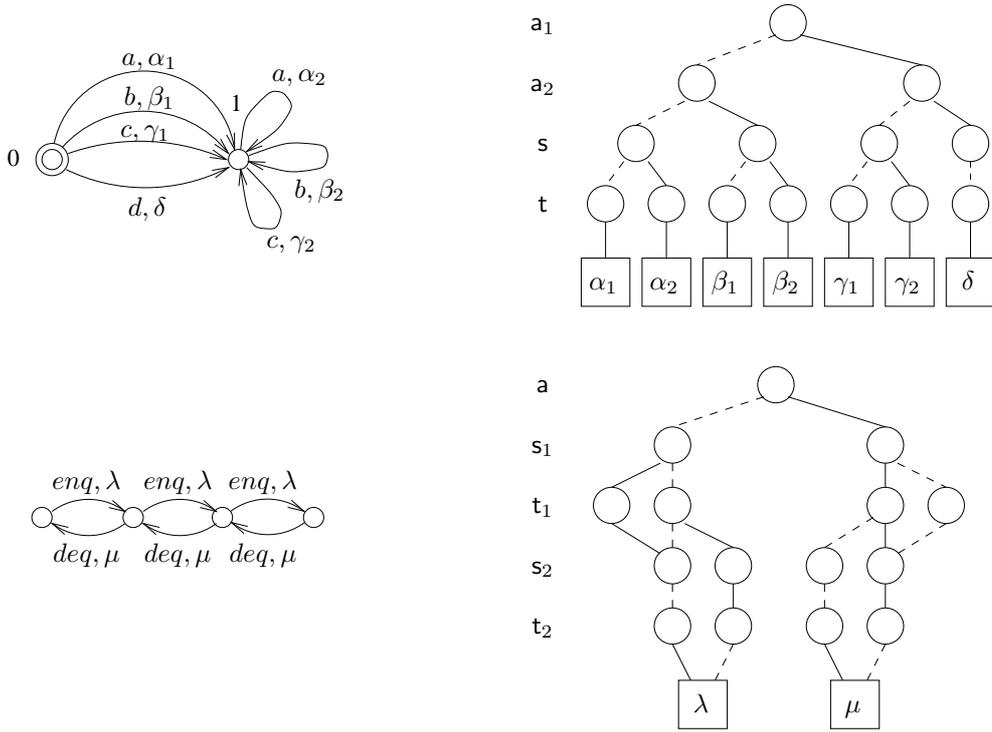
Figure 4.12: SLTSs and corresponding MTBDDs
