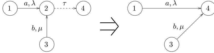
Figure 5.8: Simple redirection of transitions
