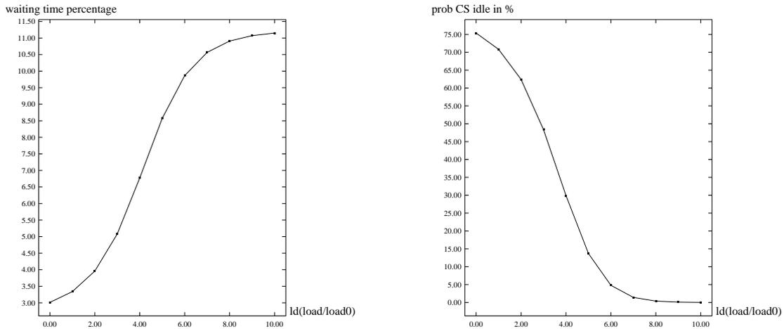
Figure 10.5: Left: waiting time percentage in subsystem MLS dependent on background load. Right: probability of CS being idle. (Note the logarithmic scale.)
