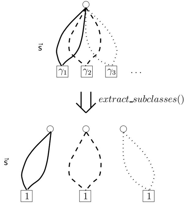
Figure 5.11: Sketch of MTBDD  $M_{cum\_rates}(\vec{s})$  (top), and effect of procedure  $extract\_subclasses()$
