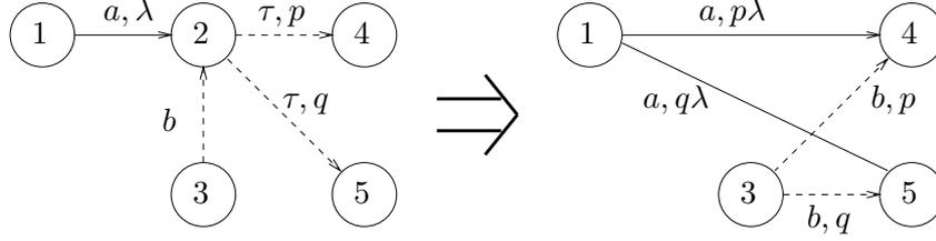
Figure 5.9: Resolving non-determinism by probabilities
