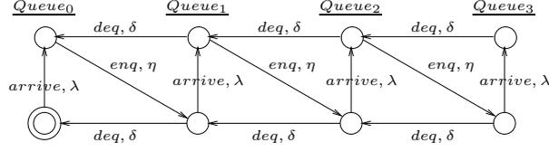
Figure 3.5: Semantic model of the Markovian queueing system, isomorphic to a CTMC
