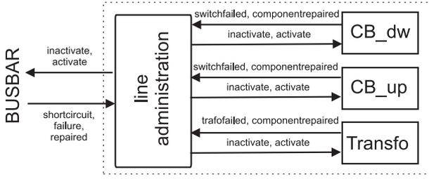
Figure 2: Sketch of the model of a trafo line
