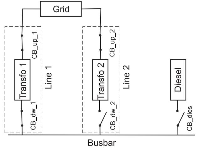
Figure 1: Sketch of the busbar model
