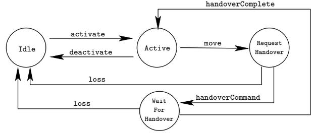
Figure 2. State machine for the MS behaviour
