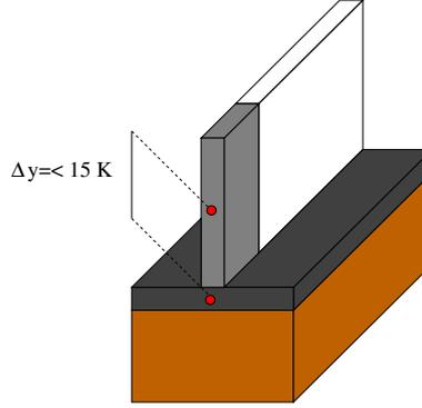
Figure 3: Geometry for the temperature criterion: Old bottom plate (black), old wall(gray), a new wall (white) and substrate (brown). The temperature difference along the middle points in  $x_2$ -direction is observed.
