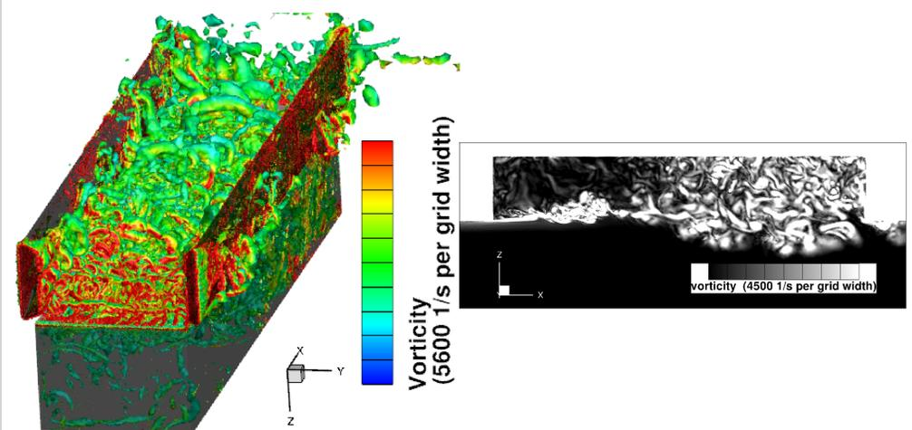
Figure 2: Shear layer instability (left) growing in its width seen in the streamwise direction (right)
