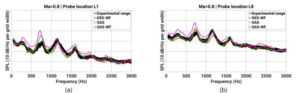
Figure 3: Spectral analysis of the pressure signal - hybrid RANS-LES and SAS approaches
