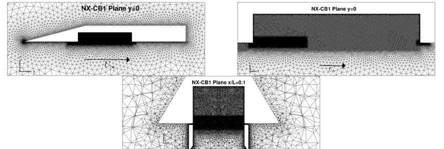
Figure 1: Mesh distribution showing fine resolution of crucial regions
