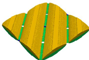
Figure 5 : Unit-cell model of the bixal carbon fabric HPT-610.
