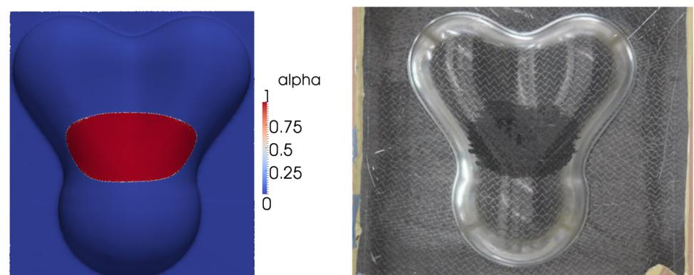
Figure 6 : Topview of the "Sattel" geometry. Simulation (left) and experiment (right) at  $t = 20s$ .
