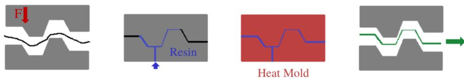
Figure 1 : Four separate phases of the RTM process.
