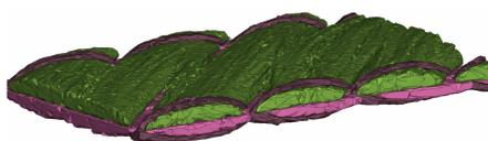
Figure 3 : Mesoscale: CT-Scan of bixal carbon HPT-610 fabric specimen by ITV Denkkendorf.
