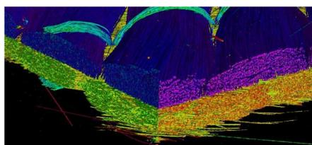
Figure 4 : Microscale: CT-Scan by ITV Denkkendorf showing filaments of a carbon fabric.
