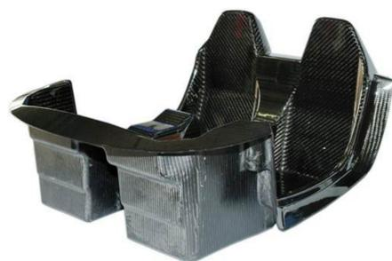
Figure 2 : Macroscale: Driver cabin completely made of carbon by SK Carbon Roding.
