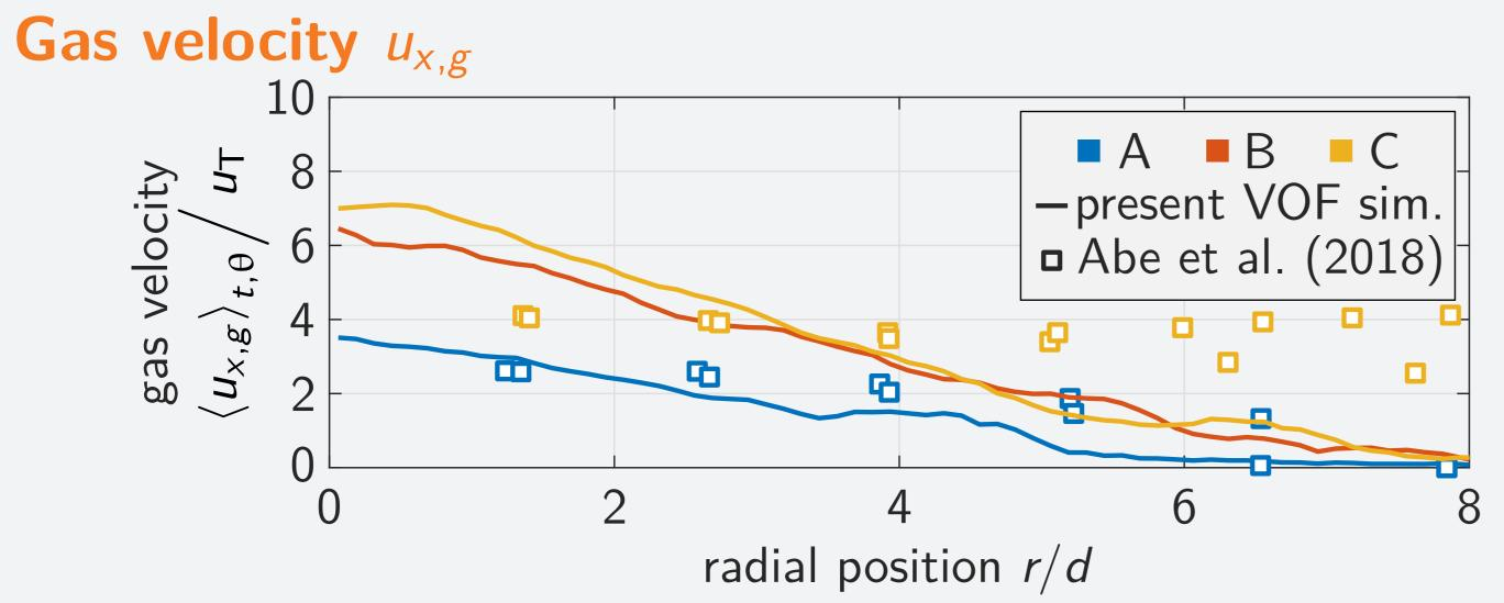
► Similar magnitude of gas velocity compared to Abe et al. (2018) at a height of x/d = 16 (no data available for case B)
