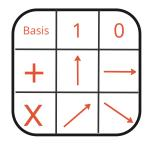
Figure 4.3: An example matrix for assigning bases and bits to polarizations
