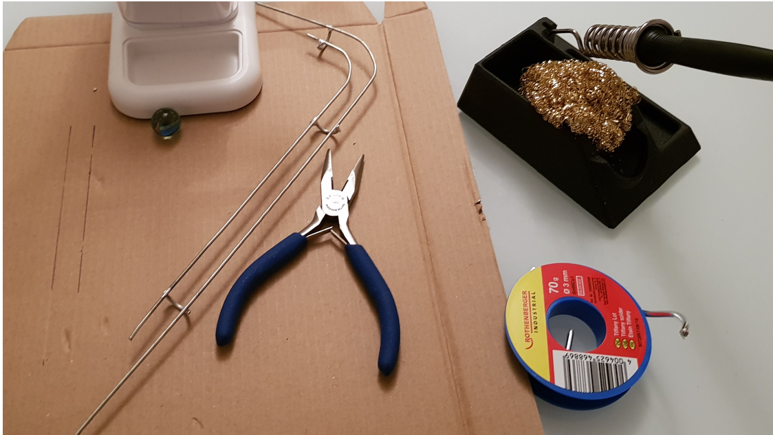
Figure 5.15.: A test track made with steel wire and solder
