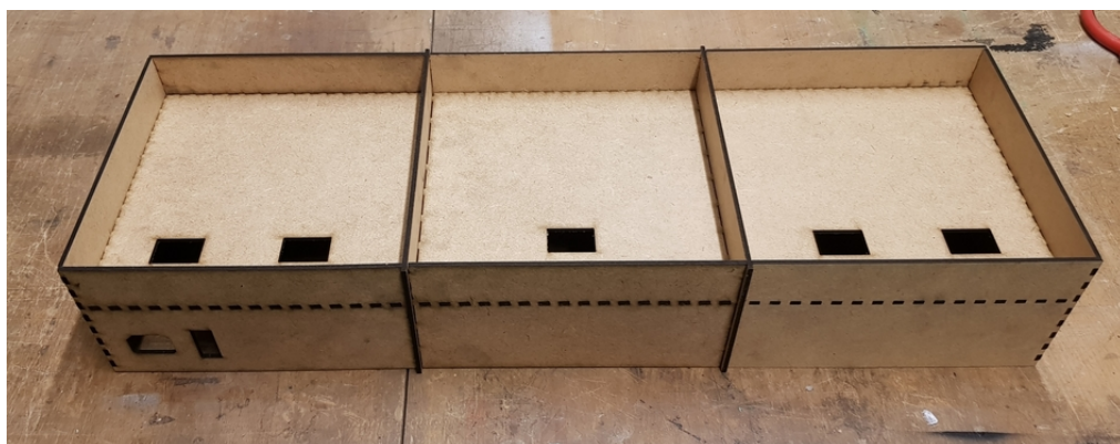
Figure 5.2.: Completed base box for the prototype
