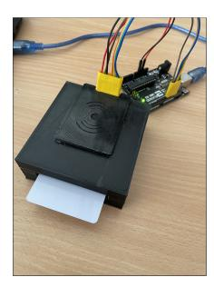
Figure 5.4: Final 3D printed smartcard reader case with inserted smartcard.
