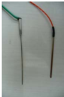
Thermoelement (grün) Widerstandsthermometer (orange)
