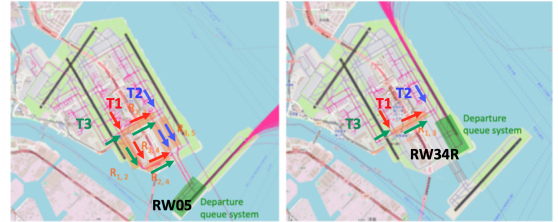
Figure 3: BSRs at RJTT. BSRs are shown in rectangles connecting BIAS with departure traffic flows from each the terminal.
