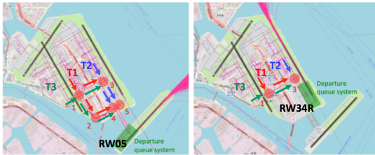
Figure 2: BIAS at RJTT. BIAS are shown in circles with departure traffic flows from each the terminal.
