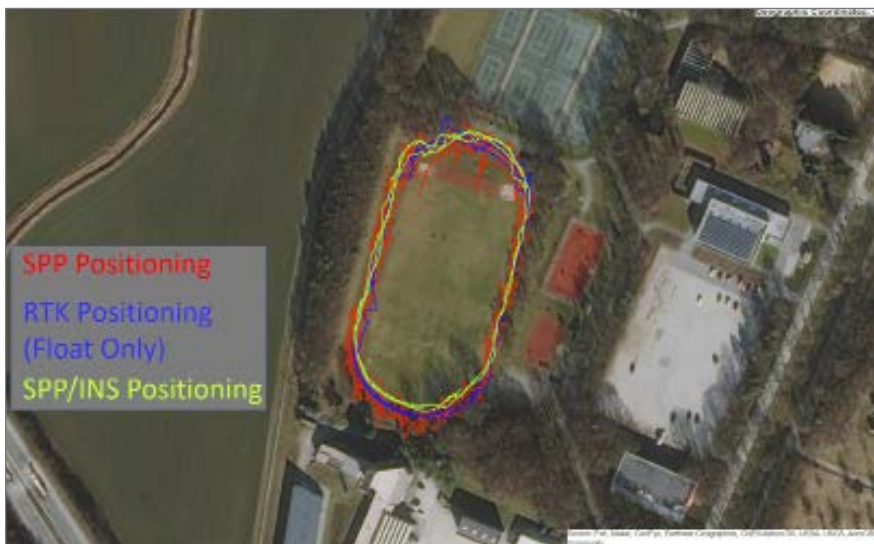
FIGURE 18 MuSNAT Analyzer UI for SPP + IMU processing Results with only SPP Trajectory (Red), RTK Trajectory (blue) and SPP/INS trajectory (green) the brown dots are the GNSS/INS Filter output positions (left) Output Map View (right), Smartphone attitude from GNSS/INS integration filter (bottom).
