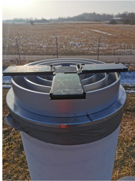
Figure 11: Experiment setup for the exact determination of the Smartphone APC location, to be interpreted from top to bottom (Left), Experimental setup with real environment conditions for Smartphone APC determination (right)
