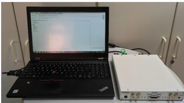
Fig. 5: NI USRP 2955 connected to a processing PC
