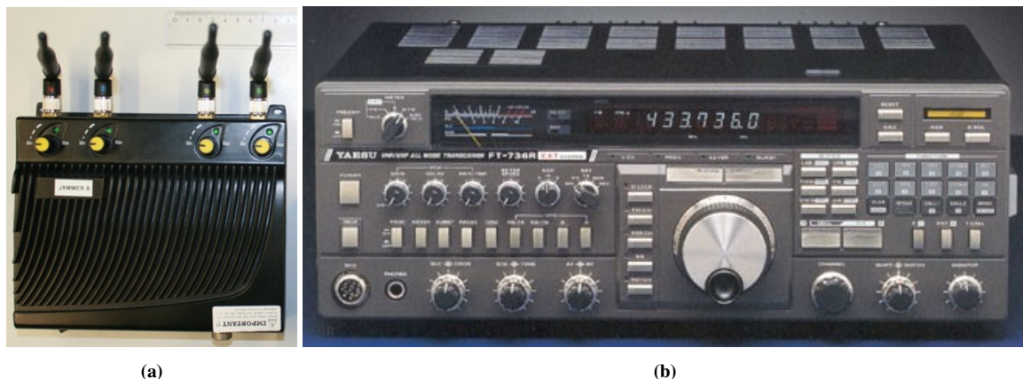
Figure 7: Used RFI for the tests: (a) Personal Privacy Device, and (b) YAESU FT-736R (FM/SSB Amateur Radio Receiver) [Source: https://www.universal-radio.com/catalog/hammulti/ft736r.html ]
