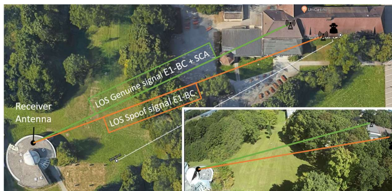
Fig. 4. Illustration of the geometrical and environmental setup of the SCER spoofing attack.
