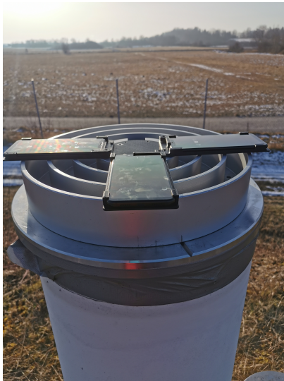
Fig. 23: Experiment setup with real environmental conditions for smartphone APC determination
