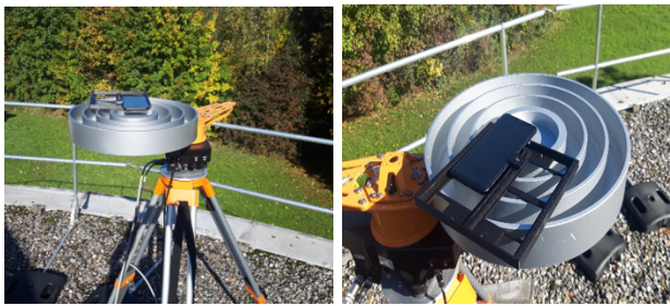
Fig. 20: Mi 8 choke-ring mounted on a rotating antenna
