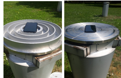
Fig. 17: Xiaomi Mi 8 smartphone with (left) and without choke-ring (right)
