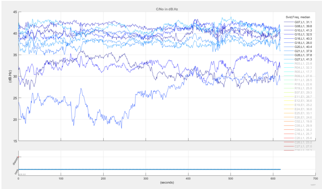
Figure 13: SNR plot for the static retransmission scenario
