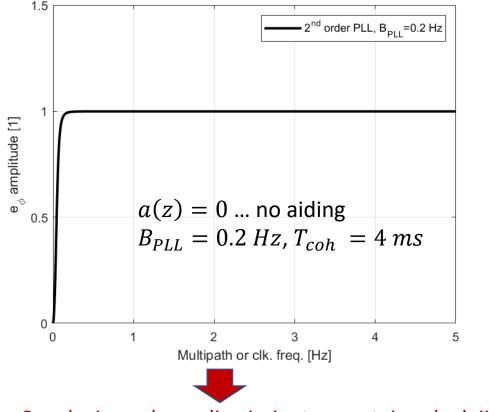
Conclusion: phase discriminator contains clock jitter, if no CoOp-aiding is applied
