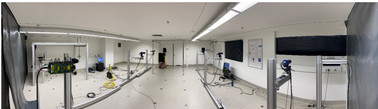
Figure 12: Optically distorted panoramic image of the test chamber with the components for the concentration measurements
