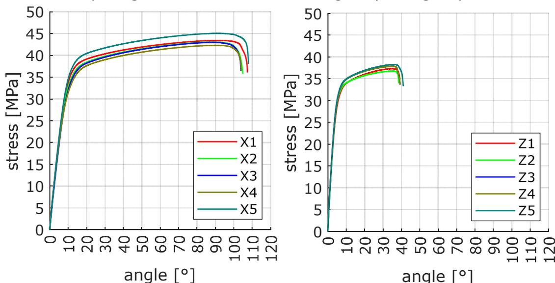
Figure 1: Results of torsional test with SLS-specimens in different orientations
