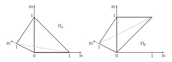
Figure 3.1: Basic reference elements for anisotropic interpolation error estimates in the three-dimensional case.
