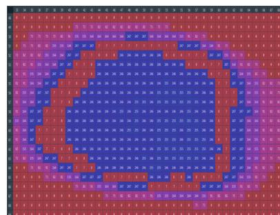
For further data processing the image will be filtered to exclude data not containing relevant information about fibers, e.g. The arrays are converted into Boolean format.
