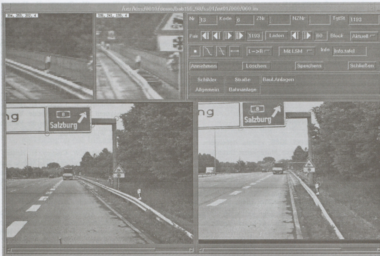
Figure 7: Object Measurement with KiSS and attributes for geographic information systems
