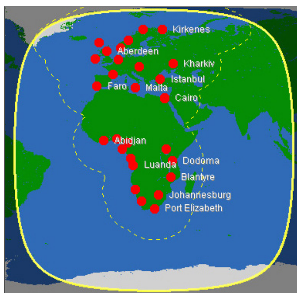
Fig. 5: OmniSTAR® coverage map for EUSAT/AFSAT from Trimble Navigation Limited [2012].
