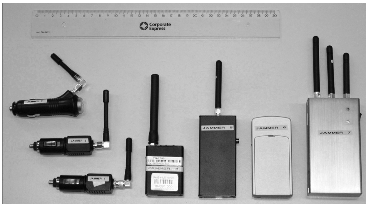
Fig. 8: Examples for commercial InCar Jammers from Bauernfeind et al. [2011].
