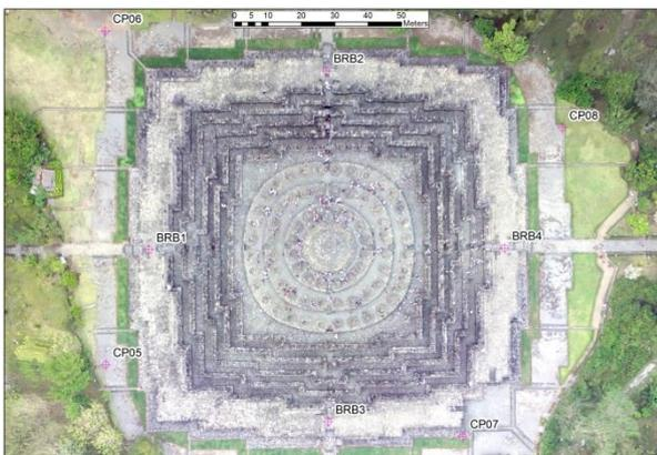
Figure 11. GCPs from GPS Survey
