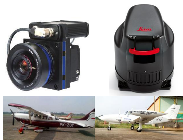
Figure 4. Aircraft and cameras used (left : Cessna 206t with Trimble P65+, right : Cessna 402b with Leica RCD30)
