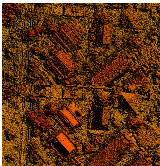
Figure 9. DSM in 10 cm GSD of BIG's office: UAV Canon S-100 (upper) and Airborne RCD30 (lower)
