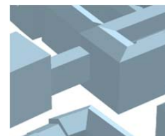
Figure 5: Not identified free hanging building in 3D city model.
