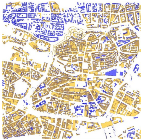
Figure 1: buildings available in OSM only (yellow), available in the the 3D city model only (blue) and in both data sets (brown).
