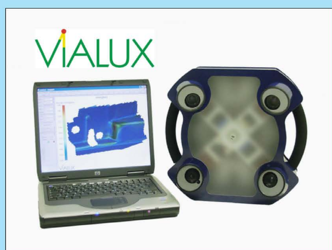
Four camera head of the VIALUX AutoGrid system for image acquisition
