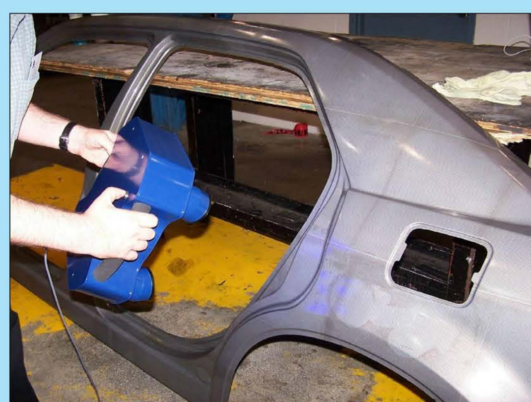
Four camera head of the VIALUX AutoGrid system for image acquisition
