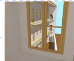
LOD 4 - Interior model walls, ceiling ... are modelled „Walkable“ architectural models
