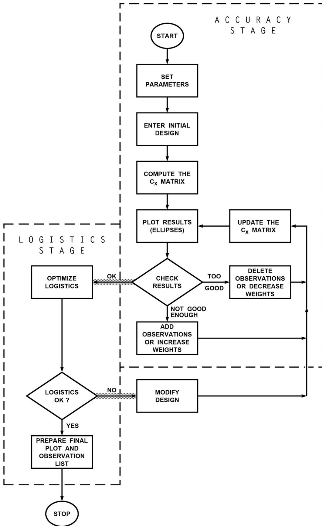
Figure 5 : SEQUENTIAL METHOD - INTERPLAY OF ACCURACY AND LOGISTICS STAGES
