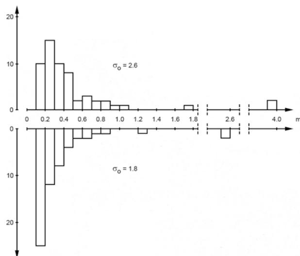
Fig. 3 - Distribution of the values of the major semi-axes of the standard ellipses for the two adjustments of net (B).
