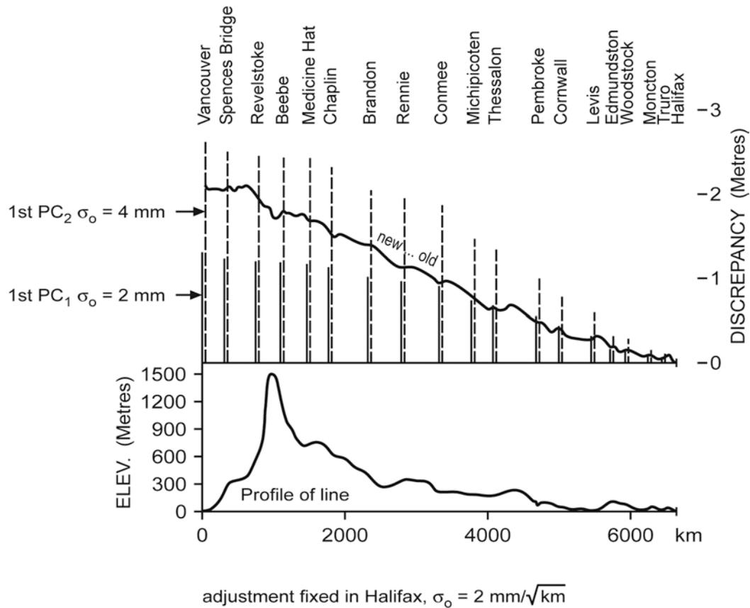
Fig. 8: Computed discrepancy for the Trans-Canada-Levelling Line and its relation to the 1st principal component.
