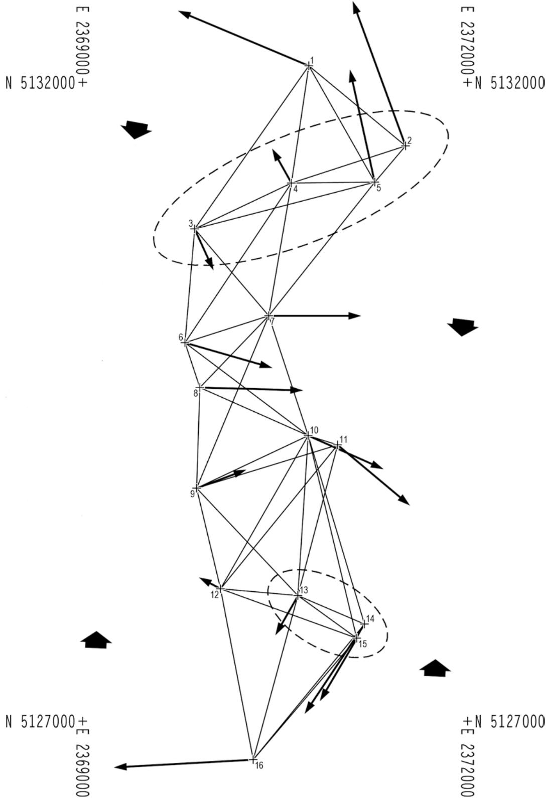
Fig. 1 Control network design to be constructed in the seismogenetic area of Friuli (Lake Cavazzo valley). The original essential eigenvector components and the predicted direction of ground deformation are also shown.
