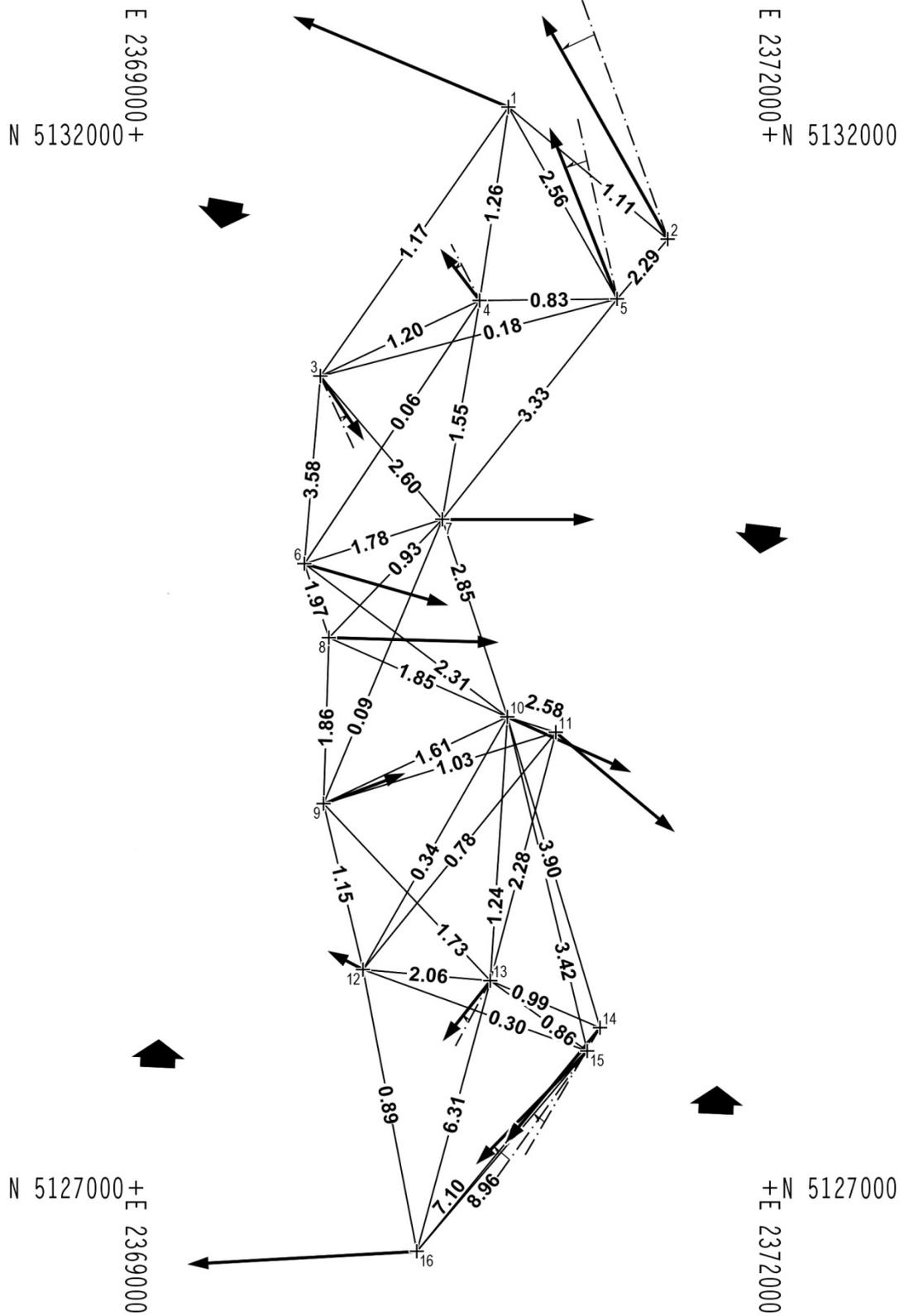
Fig. 2b Weight distribution of the observations calculated by the Second Order Design considering the matrix  $\tilde{Q}_{PT}$  as a criterion matrix.
