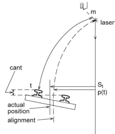
The difference  $p(t) - S_t$  is passed to the automatic guidance mechanism, which shifts the track over this distance.
