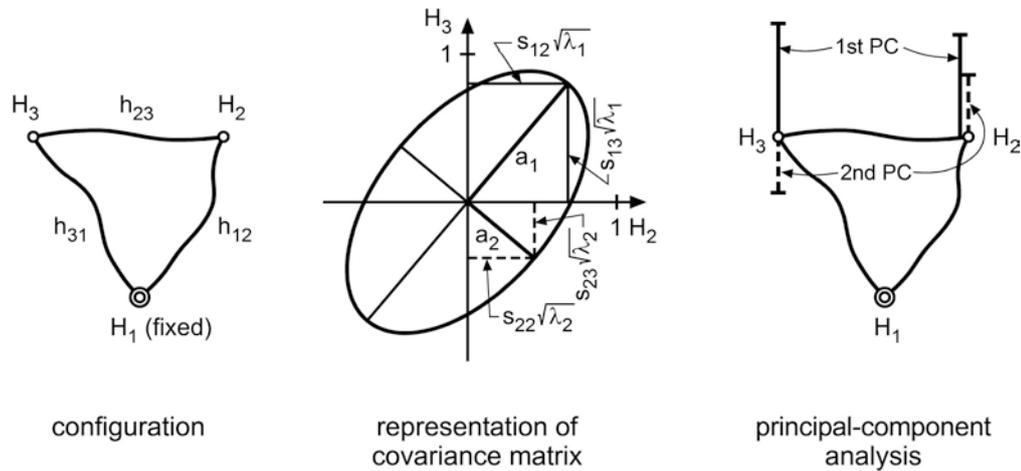
Fig. 4: Principal components for a simple levelling net.
