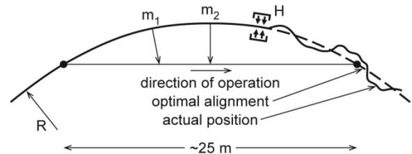
Subsequently the displacement of the track and the improvement of the cant are carried out by hydraulically operated machinery. This process is repeated from sleeper to sleeper, reaching a speed of about 0.5 km/hour. The optimal position, over which the leading point is guided, was determined up to now by one of the classical methods of measurement of "versines",  $p$ , from which the displacements  $v$  between actual and optimal position are derived in each measurement point (see fig. 3).
