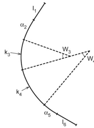
The misclosures  $q^i$  of the condition equations are functions of the parameters and of co-ordinates and bearings ; see fig. 12.
