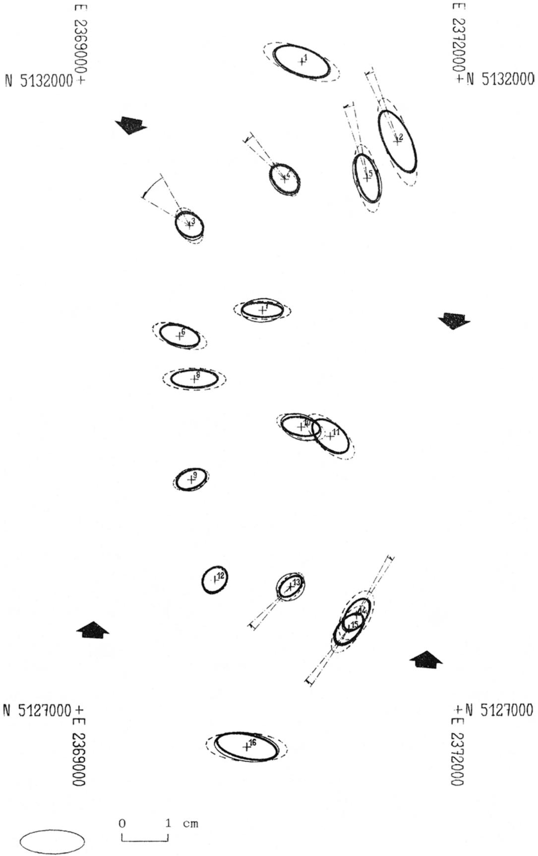
Fig. 4 Error Ellipses obtained from a unit weight matrix of the observations (dotted line), criterion matrix  $\tilde{Q}_{PT}$  (thin line) and the S.O.D. covariance matrix (thick line).
