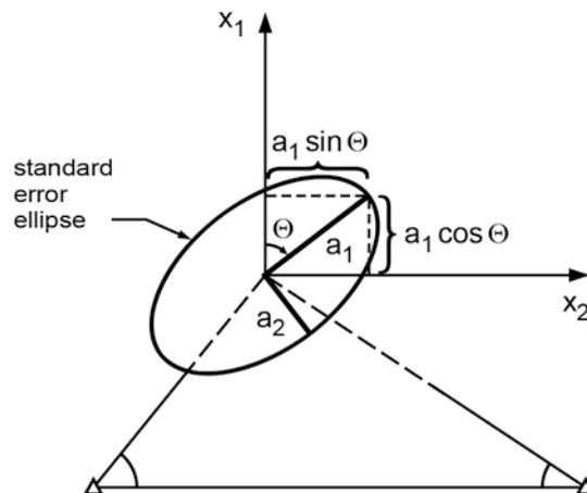
Fig. 3: Error ellipses and principal components for a point intersection.
