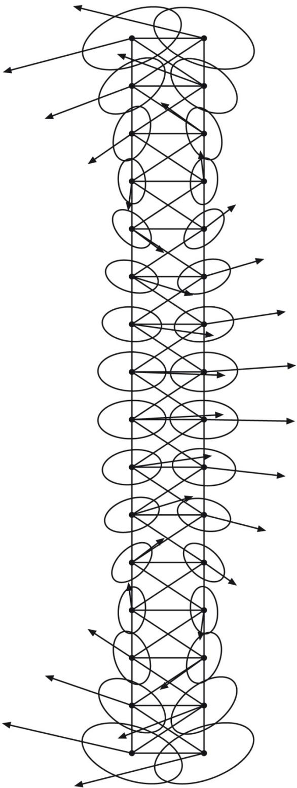
Fig. 5: Confidence ellipses and 1st principal component of a regular horizontal network (Gutberlet 1982).
