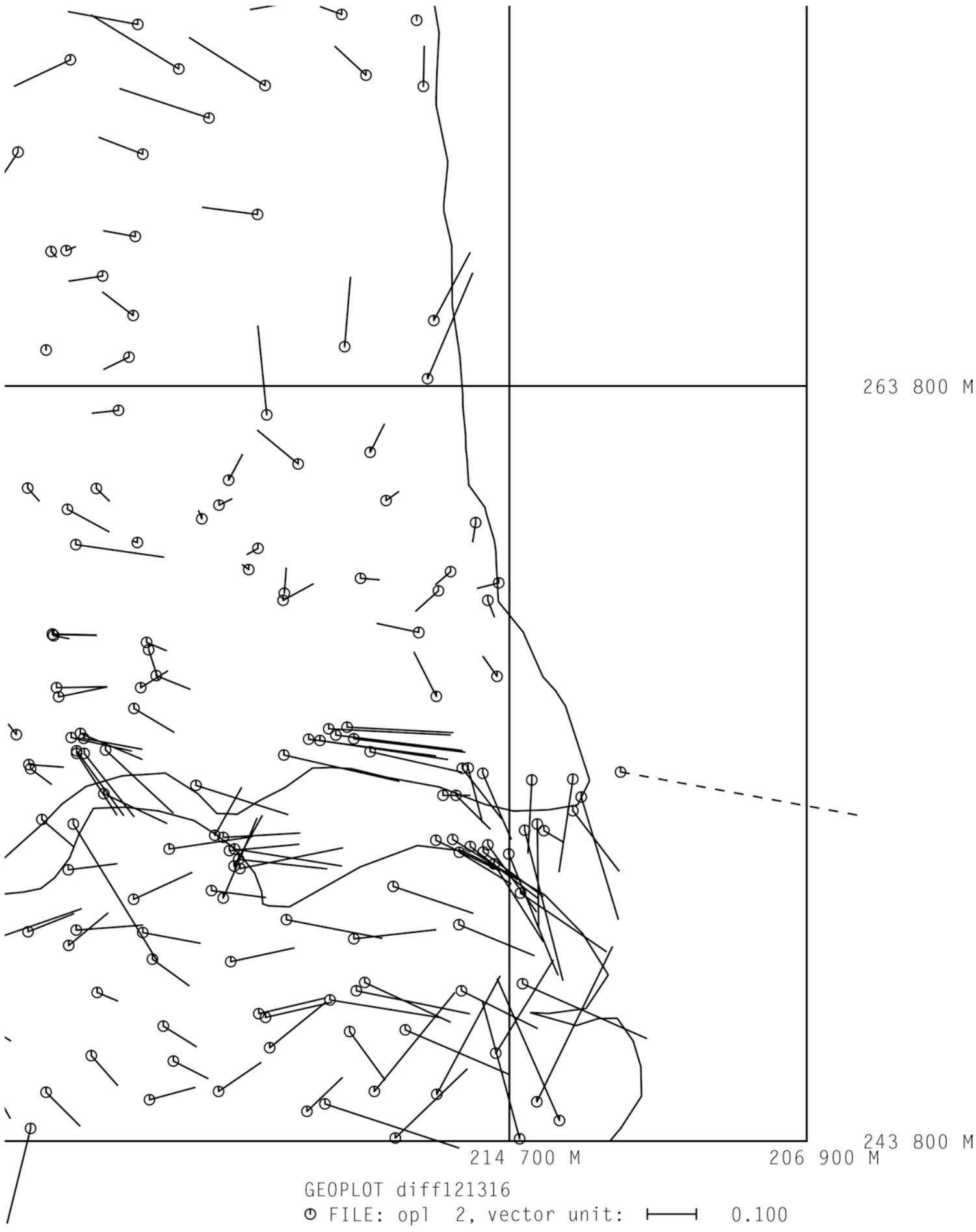
Figure 5: Section of displacement vector diagram.
