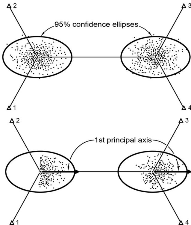
Fig. 7: Simulation study with 1000 adjustments and its relation to the 1st principal component.
