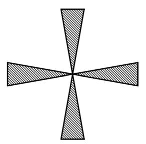
Fig. 6.5 The cross-like target, suited for oblique photos in varying scales
