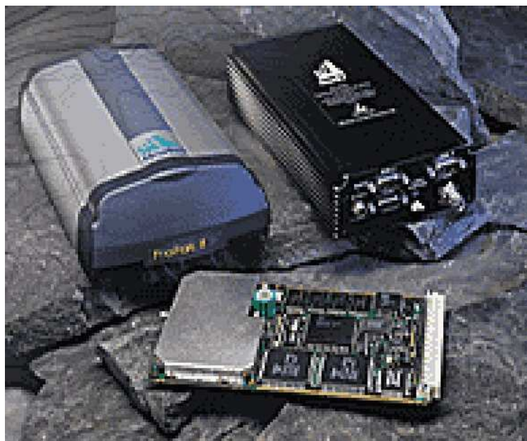
Figure 3.17: NovAtel MiLLEnium-GLONASS GPS/GLONASS receiver OEM board (taken from ( NovAtel, 1998a )).
