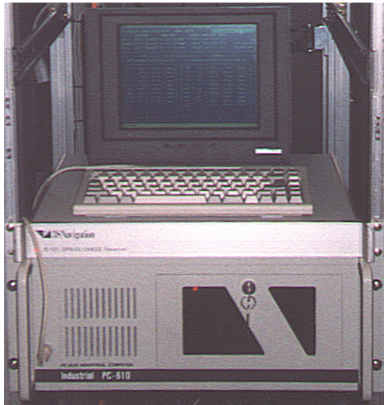
Figure 3.13: IfEN's 3S Navigation R-100/R-101 GPS/GLONASS receiver, mounted in a 19" rack.
