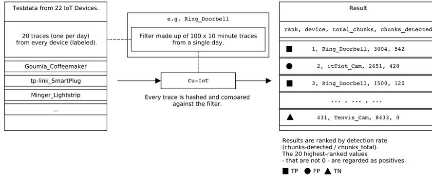
**Fig. 1.** Evaluation setup of the first and third dataset: Testrun with Ring\_Doorbell as filter device. For the third dataset the calculation ( $\text{chunks detected} / \text{chunks total}$ ) is ignored and results are ranked according to how much of their chunks were recognized overall.
