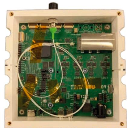
Compact transmitter electronics in a 3D printed case.
