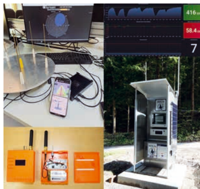
Demonstrator for the localization of LoRa transmitters with route planning to its location (top left); Excerpt of data analysis for flash flood detection (top right); ROLORAN prototype „LoRa Field Testing Device (LoRa FTD)“ (bottom left); Energy-autonomous MERLIN base in Neuhaus (bottom right).
