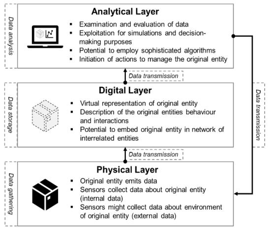
Figure 5. Basic Digital Twin architecture
