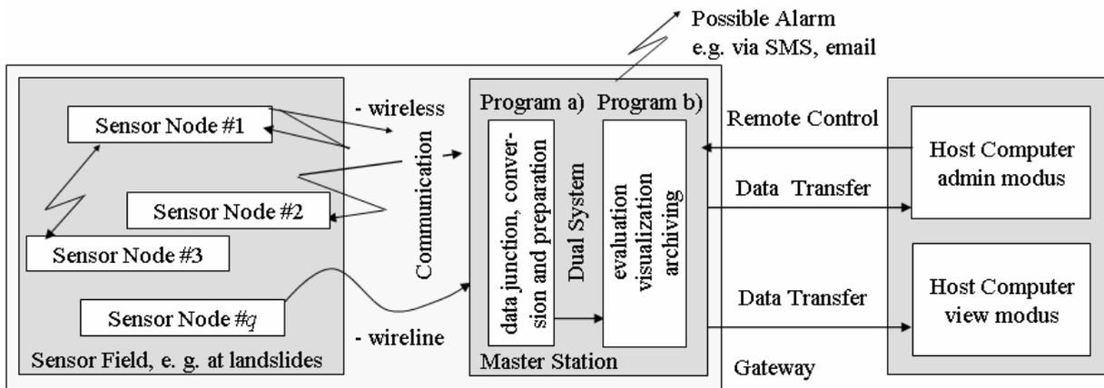
Figure 2: Basic scheme of a monitoring geo sensor network
