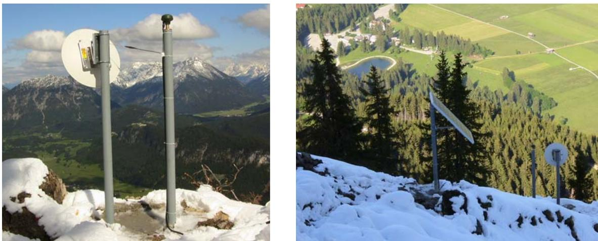
Fig. 10: Impressions from the Tyrolean Alps near Reutte at an altitude of approx. 1700 m: GNSS sensor nodes equipped with Novatel Smart Antenna, WLAN beam antenna and solar panel.
