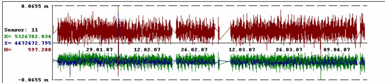
Fig. 5: Variations of a 795 m baseline (15 min. solutions) between January 15<sup>th</sup> and April 17<sup>th</sup>
