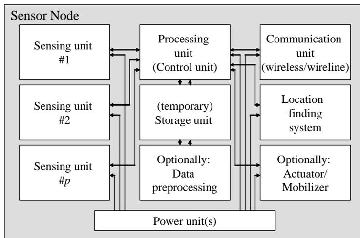
Figure 1: Typical sensor node design
