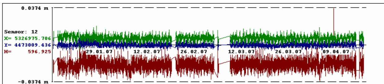
Fig. 6: Variations of a 265 m baseline (15 min. solutions) between January 15<sup>th</sup> and April 17<sup>th</sup>
