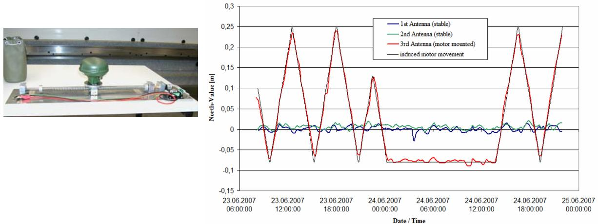
Fig. 9: Motion device (left) and comparison "true" vs. "measured" displacements (right)
